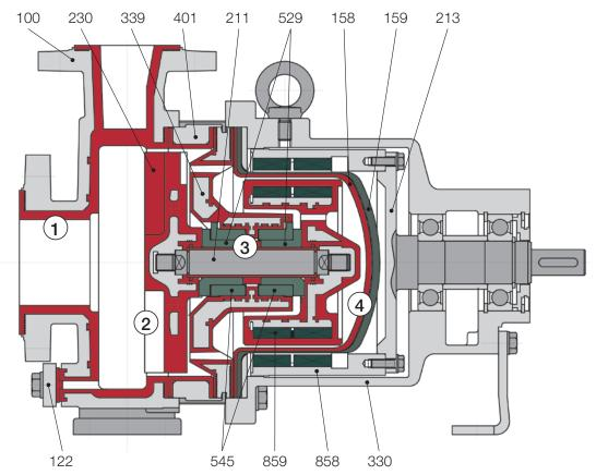
Vortex pump MNK-X with magnetic drive, frame-mounted design (alternatively close-coupled design MNK-XB up to size 80-50-200). In the event of higher solids content, flushing of the can chamber must be provided (not illustrated here, see cover photo and publication No. 657).
