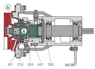
Series SCK-X with internal non-metallic double mechanical seal
